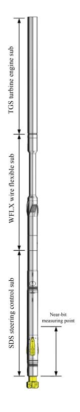
Send the ground control instruction to downhole via program-controlled shunting device CDL. Welleader® analyzes and implement the instruction through detecting the changes in mud displacement. The instruction could be sent down to the well while drilling, without affecting the drilling time-efficiency.
