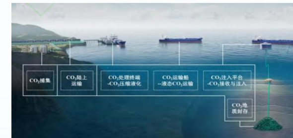
Diagram of land-to-ocean carbon transfer technology
