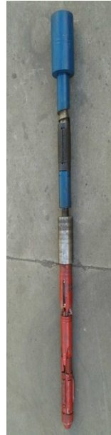
Cutting and fishing assembly
