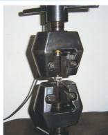
Single welding point strength test of WWS
