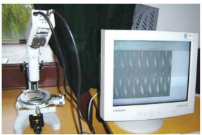
Filtration rating test of metal mesh
